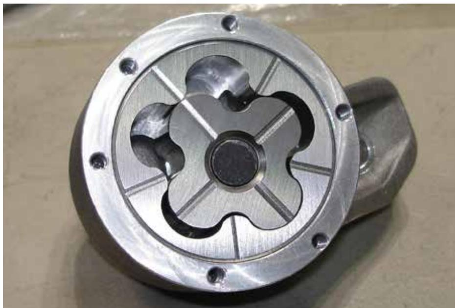
**Gerotor pumps are more cavitation resistant than straight cut spur gear pumps and produce fewer pressure pulsations** (courtesy of Schumann Sales & Service).
