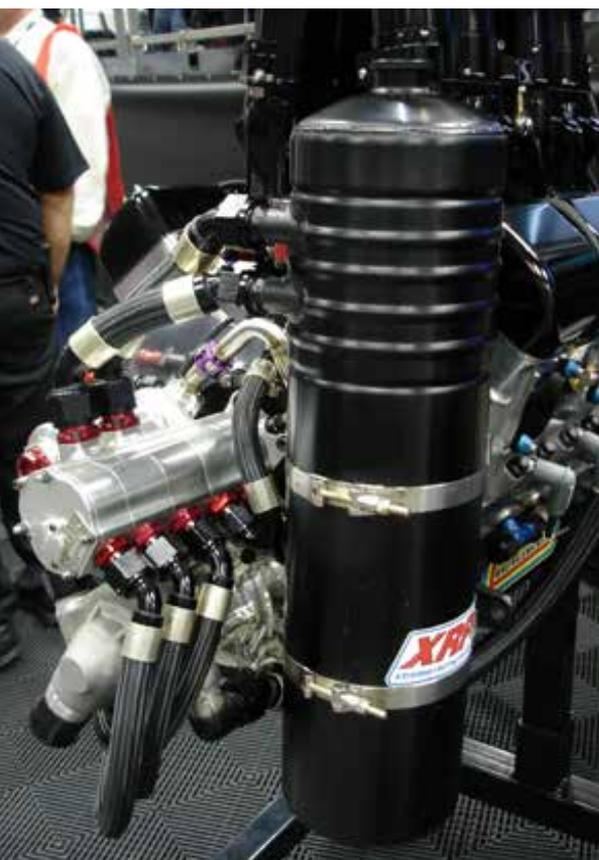
**Dry sump systems with multi-stage suction pumps pull oil out of the crankcase, separate oil and air and maintain a steady oil supply to the engine.**
