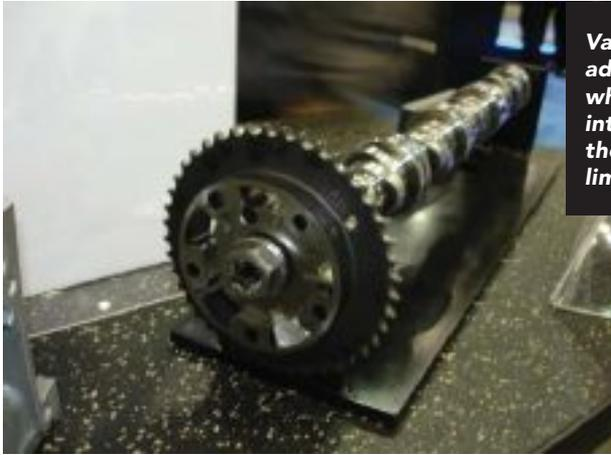
*Variable valve timing can advance or retard cam timing, which may lead to valve interference problems unless the cam phaser is locked or limited.*
