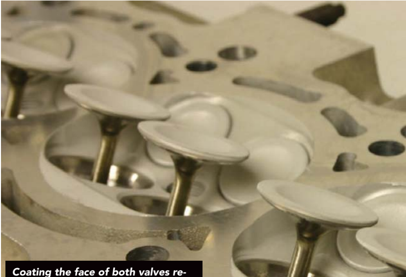
Coating the face of both valves reflects heat back into the combustion chamber and helps the valves run cooler (especially exhaust valves).
